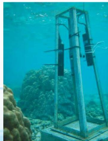
The iSAMI analyser was deployed in the lagoon of Albion. This equipment provides high resolution in-situ pH measurements
