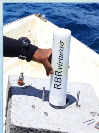
Figure 28: Pressure sensor wave recorder deployed at Albion.
