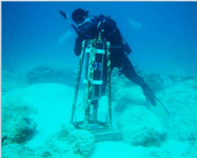
**Figure 35: ECM deployed at 6.5m depth.**
