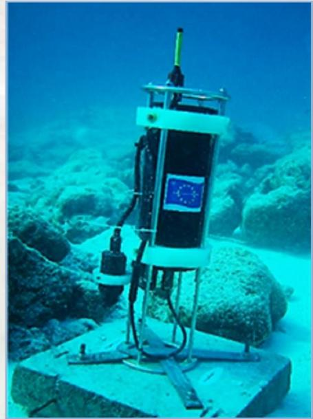
**Figure 34: CTD deployed at 6.5m depth.**
